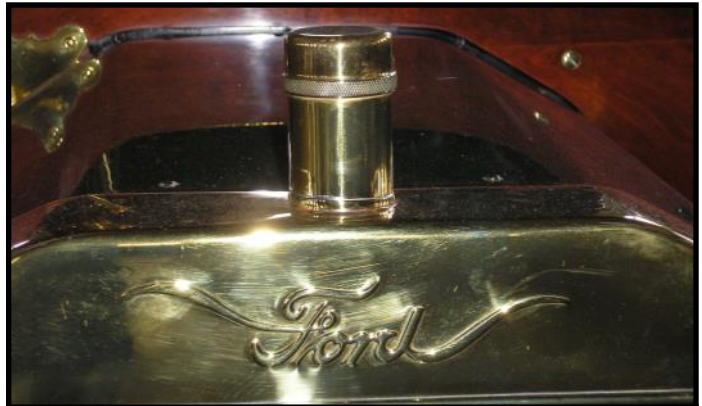
Ford Model Ts built at the Piquette Avenue Plant can be identified by the flourished "wings" on the Ford script on the radiator
