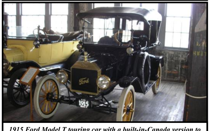
1915 Ford Model T touring car with a built-in-Canada version to its left—note the left front door not present on American cars
