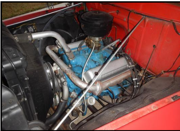
The F-100's original 239-ci Y-block V-8 engine
