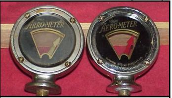
Front and back of Aero-Meter radiator temperature gauge
