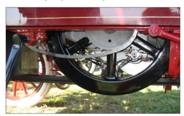
No starter motor—it took brute strength to spin the crank which is connected by chain to the huge flywheel of the single cylinder engine. This really is a get-out-and-get-under car.
