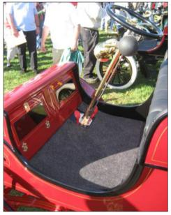
The dash has a glove compartment. The matching plate in front of the steering wheel does not open. The break pedal is on the right and the low speed pedal is on the left. The bulb horn was a necessity when roads were meant for wagons and horses, not cars.
