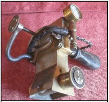
Early Harvey Frost vulcanizing device. A real "Rube Goldberg" contraption fueled with gasoline fire to produce steam heat.
