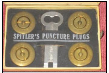
Brass "puncture plugs" designed to screw into a tire casing to plug a hole. Installation tool included. This NOS set was a gift to Terry from the late Merritt Horne, founding member of the TRAACA.
