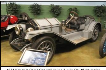
1912 National Speed Car with inline 4-cylinder, 40-hp engine
