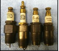
A few of the spark plugs designed specifically for the Ford Model T
