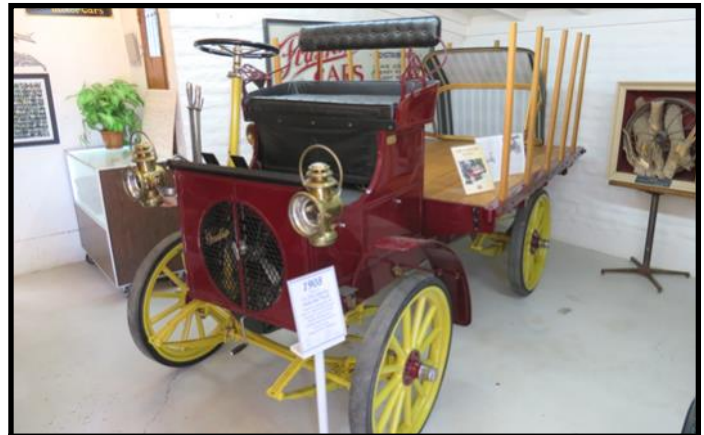
1908 Franklin Model J 1.5-ton capacity Stake-Bed Truck
