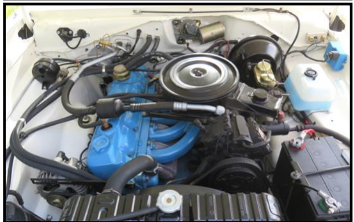
The Scamp's powerful 105-hp, 225-ci "Slant Six" engine
