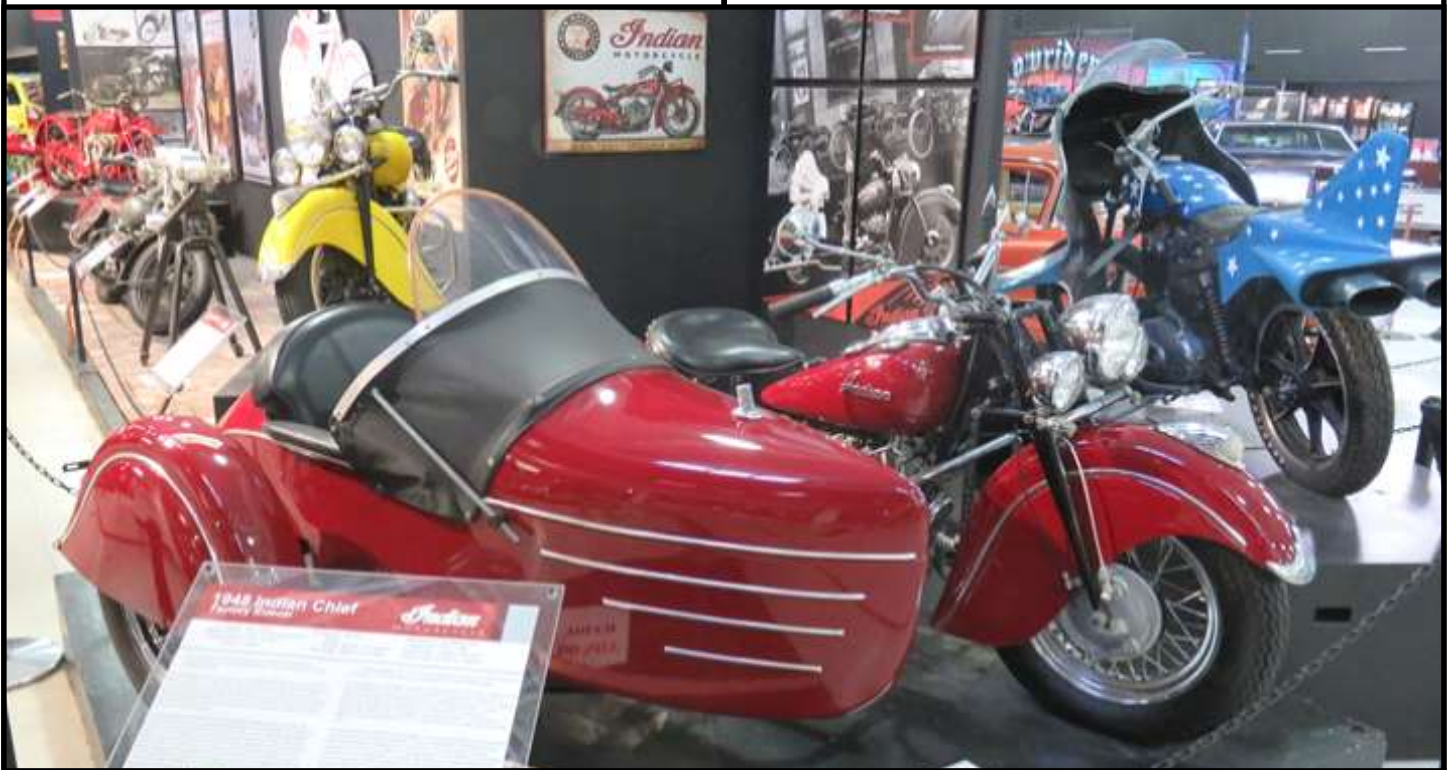
1948 Indian Chief motorcycle and sidecar—the sidecar had its own brake to help stop the combined weight of 800 lbs plus driver & passenger
