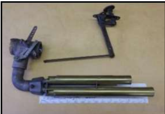
An example of an Aermore type exhaust whistle showing mounting hardware.
