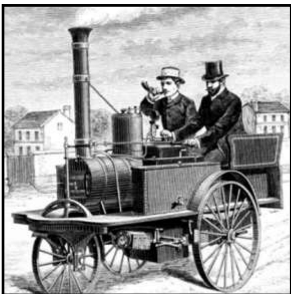
An early illustration of a steam-powered vehicle showing a trumpet used as a warning signal.
