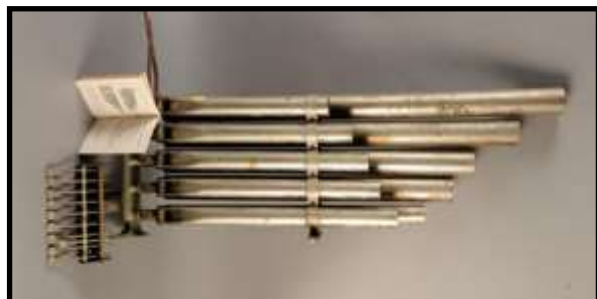
A ten-tube Gabriel exhaust whistle complete with keyboard and instruction sheet.
