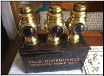
"Get you home" kerosene lamps in case the electrical system fails
