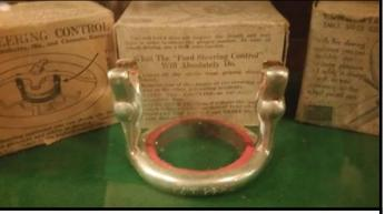
A Ford Steering Stabilizer, designed to eliminate vibration in the steering wheel
