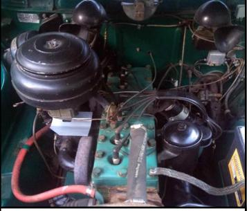
CORRECTION: In the July Mudflap the caption on the engine for Bruce Sedel's 1949 Studebaker Commander was incorrect. The engine was increased in 1949 to 245-cubic inches & 102 horsepower.
