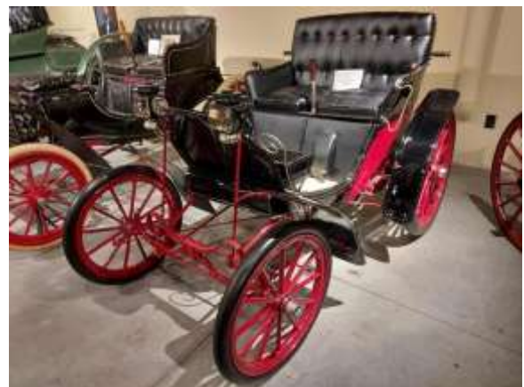
1903 Duryea. Note the “joy-stick” style steering and control lever in the center of the seat.
