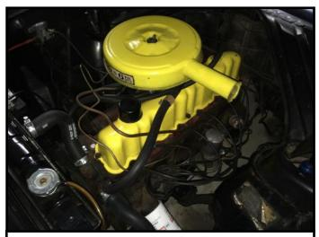
The Comet's original 260-cubic inch straight six-cylinder engine
