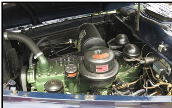
The Packard's 356-cubic inch, 165-hp, straight 8-cylinder engine
