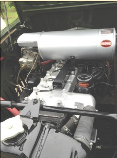
Left: The 323 c.i. straight eight with aluminum Silver Dome cyl- inder head.
