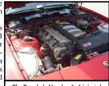
The Porsche's 16-valve, fuel-injected, 188-hp 2.5L inline 4-cylinder engine
