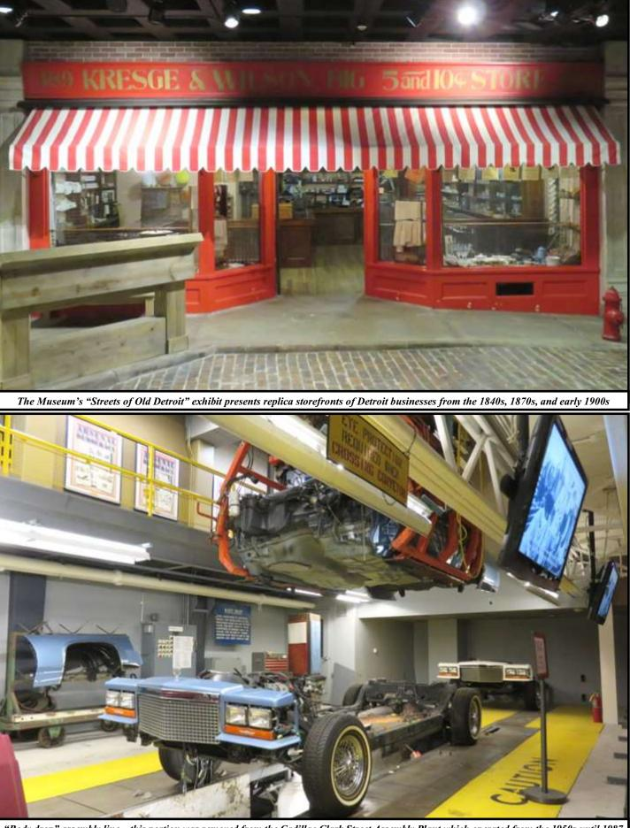
"Body drop" assembly line—this portion was removed from the Cadillac Clark Street Assembly Plant which operated from the 1950s until 1987
