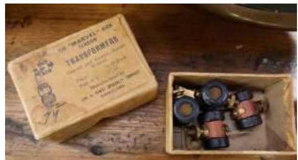
These accessory spark intensifiers were sold to help prevent oil fouling your spark plugs. They are not only interesting little gadgets, they fit very well with my spark plug collection!
