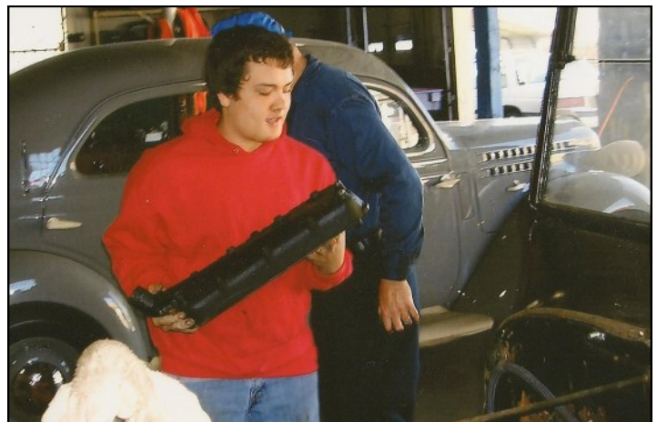
Tyler getting ready to re-install the Model T's cylinder head. The engine had been locked up for years, and required a re-build to run again.
