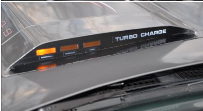
The Trans Am features a turbo light turbo boost indicator set in the shaker-style hood.
