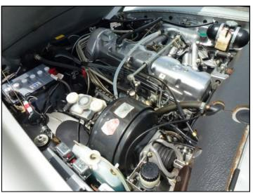
The 2778cc 6-cylinder engine produces 170 horsepower. Each engine was bench-tested for two hours before being fitted.
