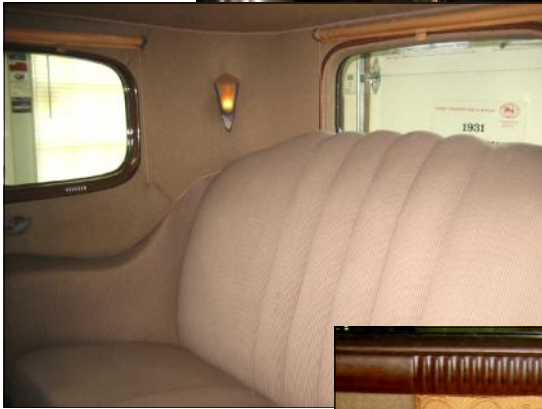
Each door has wood grained molded trim over a brocade panel. Note the styling of the doorknob base.
