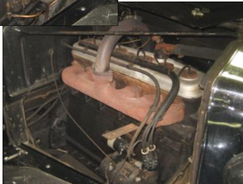
Curved pipe over the engine is the exhaust manifold which goes past the carburetor to provide carb heat
