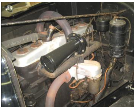
Willys-Knight engine showing horn, carburetor, and vacuum tank
