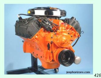
hemi, note spark plugs in center of valve cover
