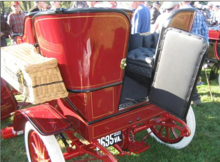
*Passengers entering the rear of the car step over a metal CADILLAC plate. The engine is under the front seat with access through the floorboard and from under the car.*
