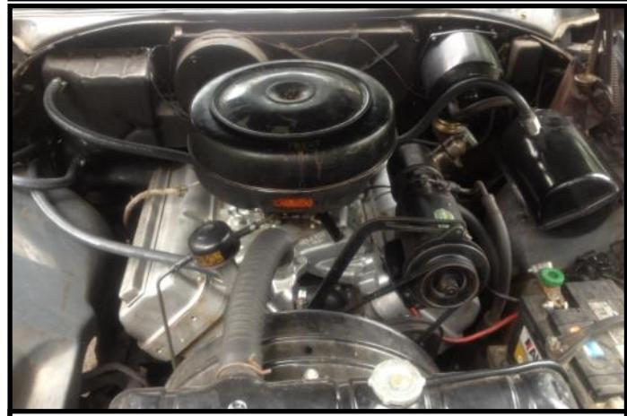
*The 1956 DeSoto Fireflight has a 330-ci, 230-hp V-8 hemi engine*
