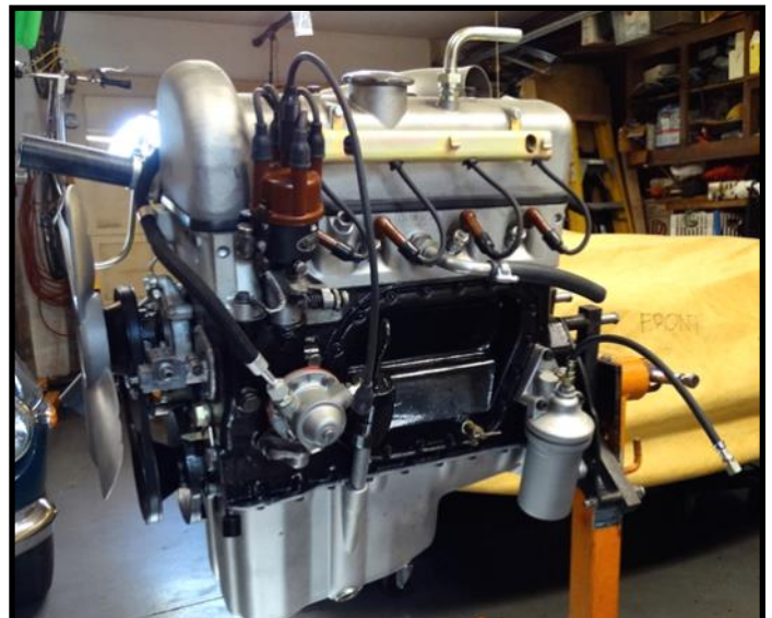
Frosty's rebuilt 1,897-cc, overhead cam, 4-cylinder engine
