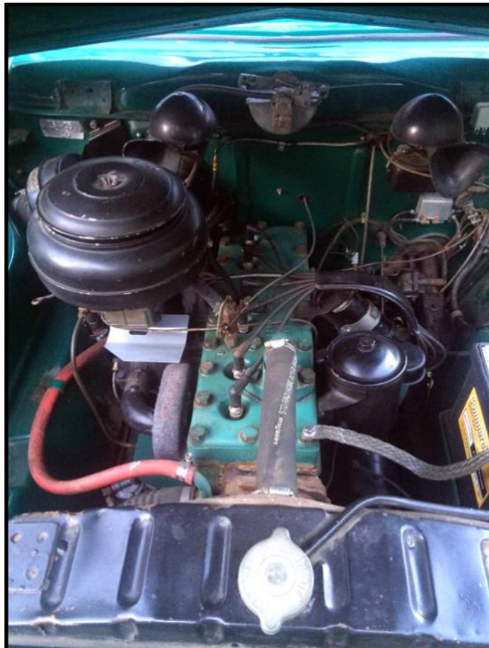
The 1949 Stude's 245-cubic inch, 102-hp, "big six" engine
