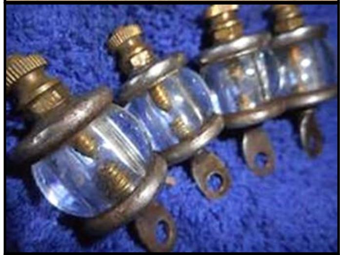
*Spark intensifiers attach to spark plugs. (These are circa 1909.) The air gap and resulting spark jump intensify the spark. Spark intensifiers were popular for older oil-burning engines.*
