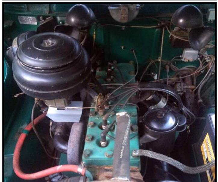
**CORRECTION:** In the July Mudflap the caption on the engine for Bruce Sedel's 1949 Studebaker Commander was incorrect. The engine was increased in 1949 to 245-cubic inches & 102 horsepower.
