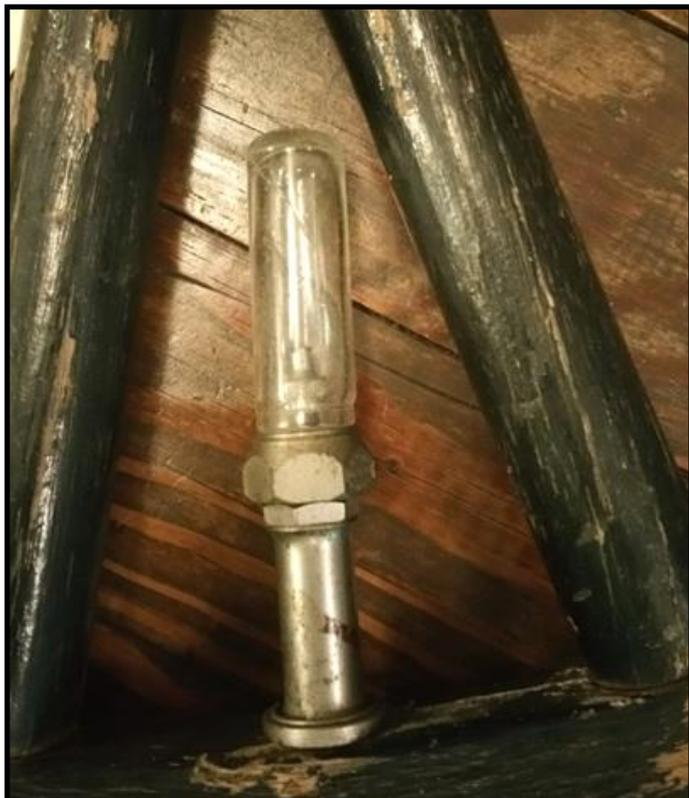
*A glass, tire valve stem cover. When these were filled with water, they revealed air leaks by the bubbles in the water.*
