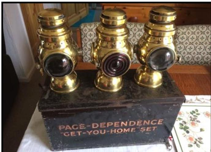
*"Get you home" kerosene lamps in case the electrical system fails*
