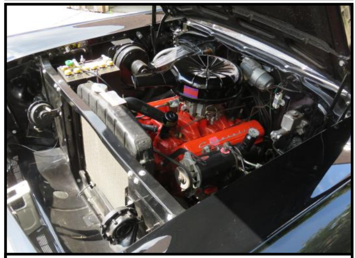
The Bel Air's rebuilt 283-ci, 220-hp, V-8 engine
