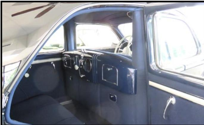
**The roll-up window separating the passengers from the driver and the backseat radio came only on Custom Berline model Cord 812s**
