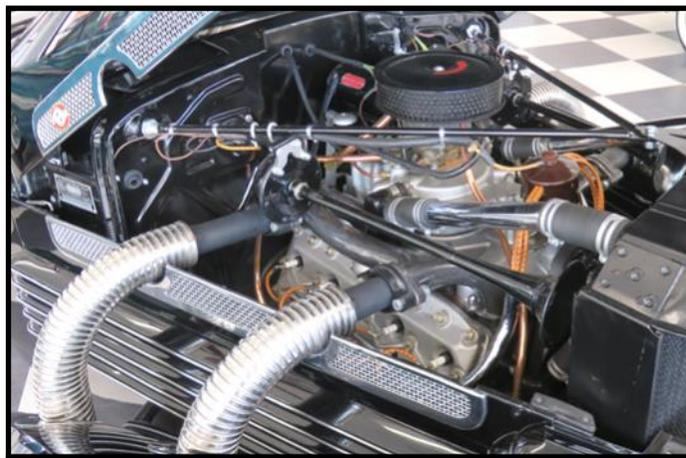
**The Cord's supercharged 289-ci, 175-hp Lycoming V-8 engine**
