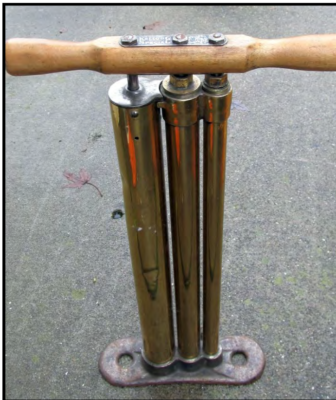
A brass triple barrel tire pump manufactured by Kellogg, a popular early manufacture of air pumps.
