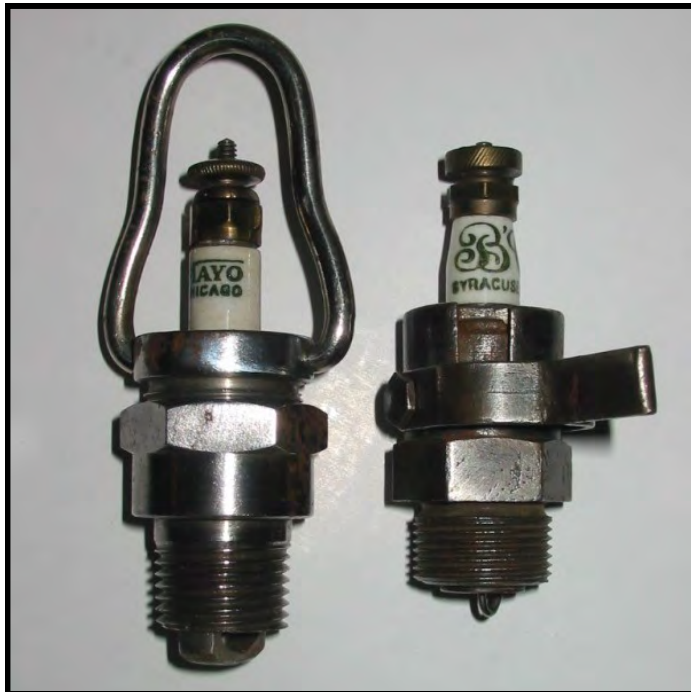
Two brands of spark plugs with removable center cores. Part of a tire pump outfit containing pump, connector, hose and inflation valve.
