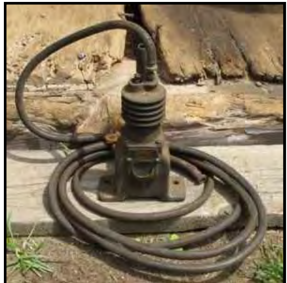
Smaller units were offered for other cars including this after-market compressor designed for the Model T Ford.
