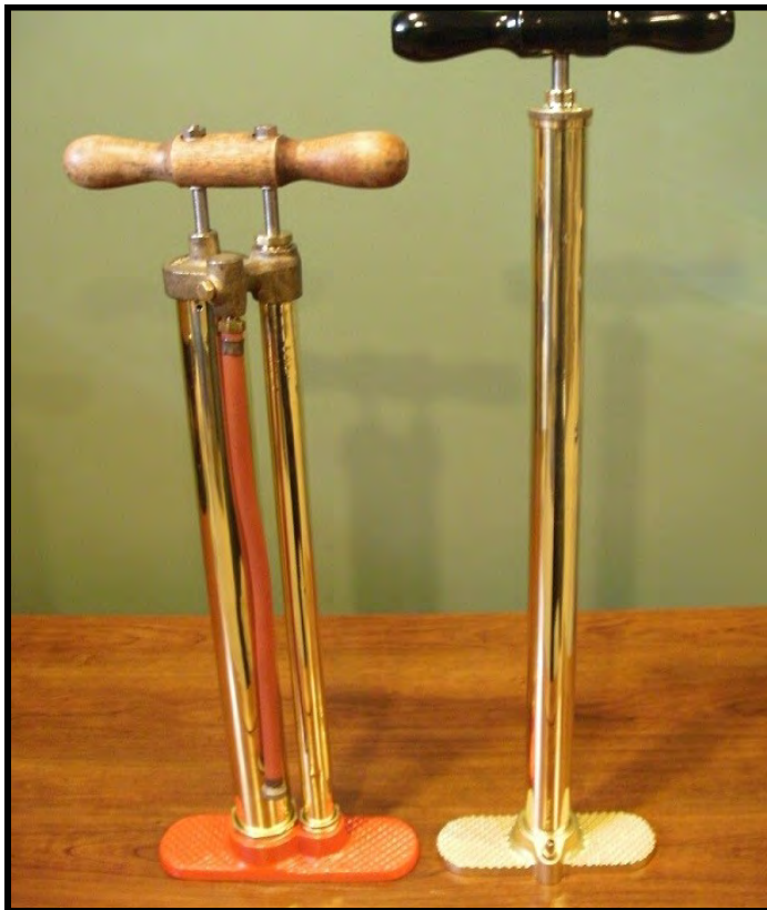
Two nicely restored early Ford tire pumps. Double, even triple barrel pumps were used to provide increased air volume.
