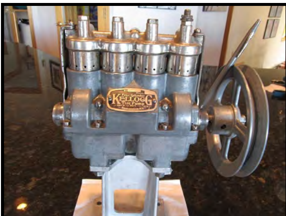
An early under-hood mounted Kellogg air compressor for easily inflating tires. One of the first car manufacturers to offer such a unit was Cadillac.
