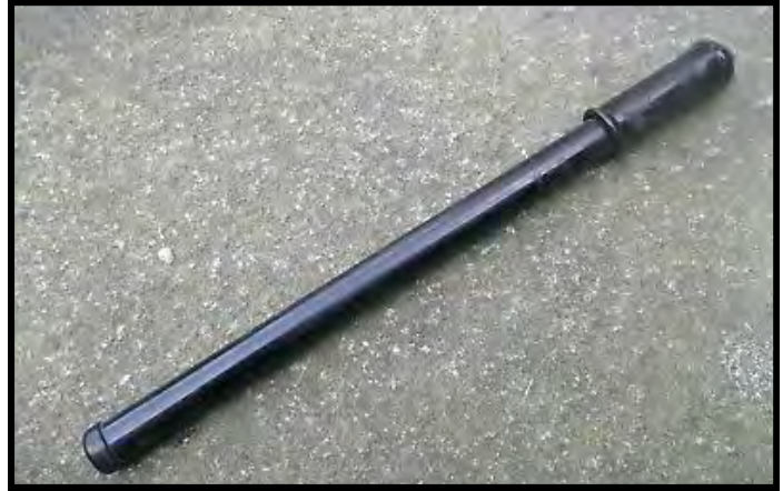
A typical early tire pump for a bicycle or early motorcycle.
