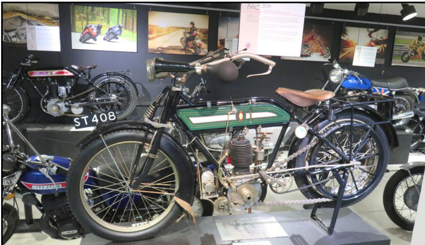
1912 BSA Model C motorcycle (with 2-speed hub and single-cylinder 500-cc engine) on display at the San Diego Automobile Museum
