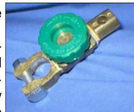
After using this on dad's Packard, I'm going to get one for the Bricklin! It sure makes it easy to isolate the battery when storing the car or working on the electrical system. The best price I've found on the unit is from Bill Hirsch
