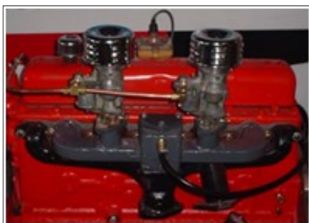
Right: Home made split exhaust and intake manifolds
