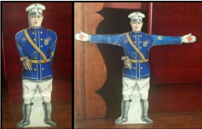
*Mounted in the rear window of a car, this policeman's arms automatically extended when the brake was applied.*
