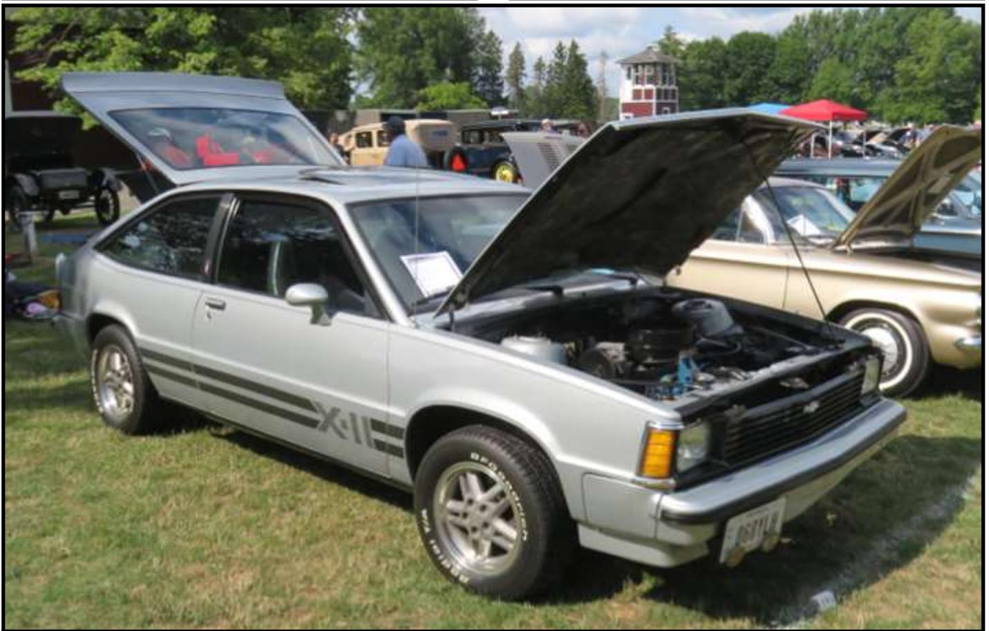
*1982 Chevrolet Citation X-11 front-wheel-drive, 3-door hatchback (with the “high output” 135-hp 2.8L V-6 engine—high-performance in the 1980s)*
