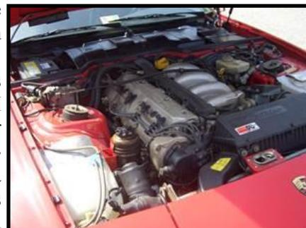
*The Porsche's 16-valve, fuel-injected, 188-hp 2.5L inline 4-cylinder engine*
